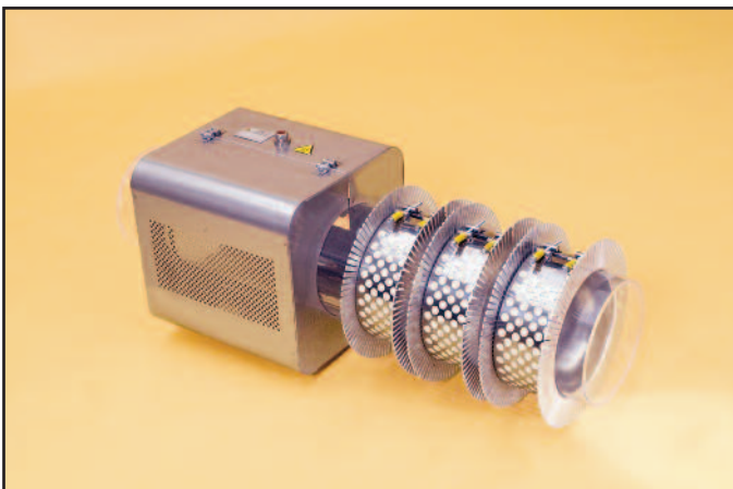
Heater bands model Z.41 with ceramic insulation with external perforated sheet. Finned dissipators (made of Al 20/10) and covering with coupling flange for blowers
